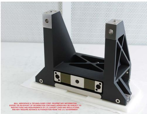
Thank you Epner for your support of the Aquila-STA Structural Mount Assembly. Your unique plating skills protected the invar and enabled the diamond turning required for this precision mounting structure's interfaces supporting the worlds highest accuracy Star Trackers.
