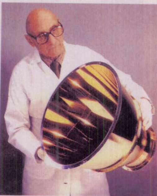
David Epner holds a cryo-radiator that was gold-coated by his company for the Canadian Space Agency's Atmospheric Chemical Experiment satellite. The spacecraft was built by Ball Aerospace.
