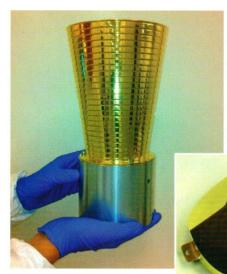
The thermal shield for the lunar corner-cube retroreflector is coated with Laser Gold to allow measurements critical in understanding dark energy and matter (inset). An additional sunshield under consideration keeps the sun off of the surface of the retroreflector for improved temperature stability. (Image credit: Epner Technology)
